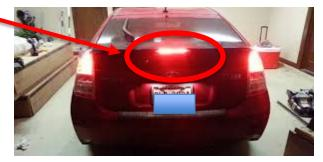
The prohibition against primary stop lamps pulsating are not applicable to motorcycles as motorcycles are not required to be equipped with *High Mount Stop Lamps*, and therefore do pulse the primary stop lamps prior to the steady illumination of the vehicle brake light if so equipped.
