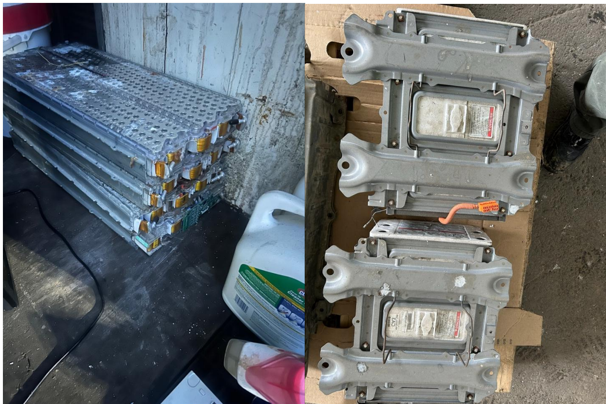
Fig. 10: Examples of stranded vehicle batteries improperly discarded at a public landfill
